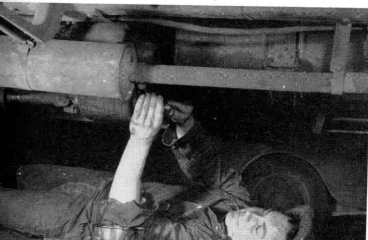
Repairing transfer case.
