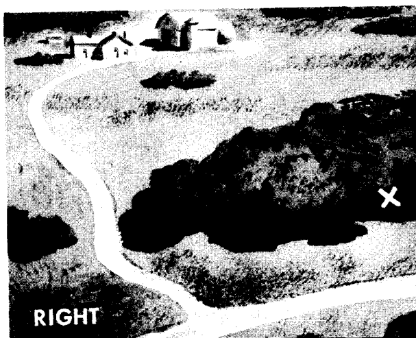
FIGURE 34. — Turn-off to installation (X) is carried beyond woods to some natural termination, such as the house, and this additional section of road must be frequently traveled so that no difference between the two sections of road is discernible.
