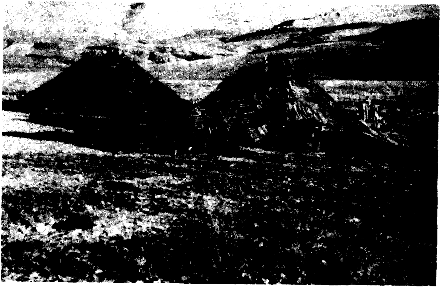
FIGURE 20.—Vehicles in barren terrain. Drapes made of garnished twine nets transform these rectangular shapes into mounds.
