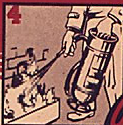
3. Turn extinguisher upside down when ready to attack fire. 4. Direct stream against inside opposite wall of container or allow foam to fall lightly on surface
