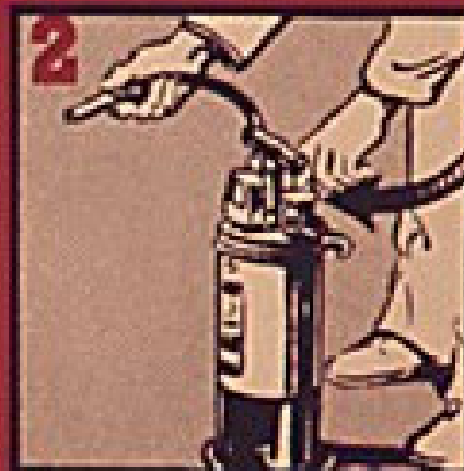
2. Set extinguisher on floor or ground, open discharge control valve B
