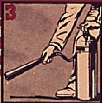
3. Loosen discharge horn—Pull locking or safety pin. Open valve. 4. Approach fire as close as possible from windward side, move horn slowly from side to side; direct discharge to base of flames, continue discharge after flame is extinguished to avoid back flash from re-ignition
