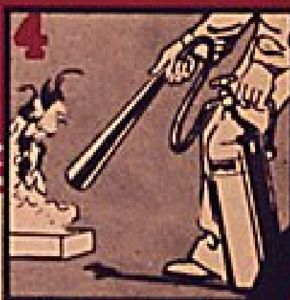
3. Loosen discharge horn—Pull locking or safety pin. Open valve. 4. Approach fire as close as possible from windward side, move horn slowly from side to side; direct discharge to base of flames, continue discharge after flame is extinguished to avoid back flash from re-ignition
