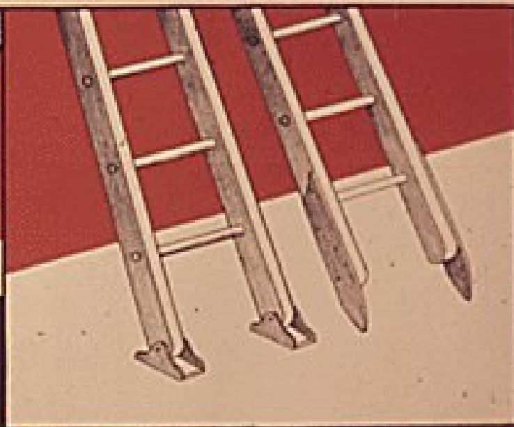
INSTALL PROPER SHOES FOR NON-SLIPPING
