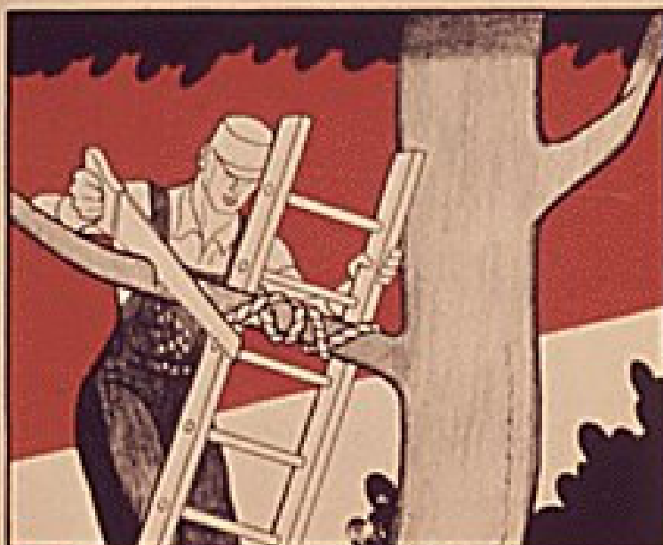
TIE TO ALL UNSTABLE SUPPORTS
